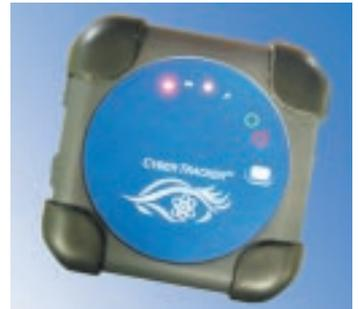
The four top buffers were combined with a sealing gasket as a single piecepart and the base buffers were produced from a 4-impresion tool to minimise costs. All of the polyurethane piece parts were produced from silicone rubber moulds, generated from SLA masters built and finished by Martello to replicate the surface texture of the ultimate production item.
